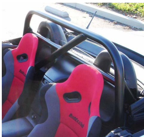
Figure 12 SCCA TTR Spec Roll Bar Honda Sports 2000 Bethania Garage
