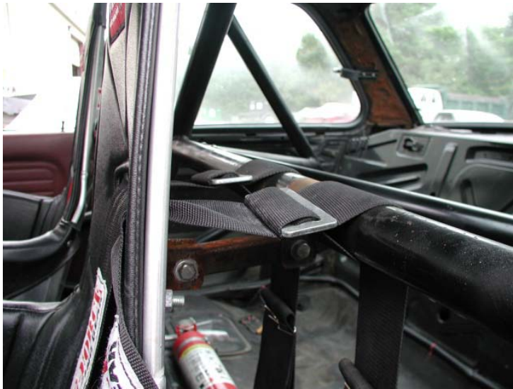
Figure 17 Acceptable Harness Bar and seat back brace mount.
