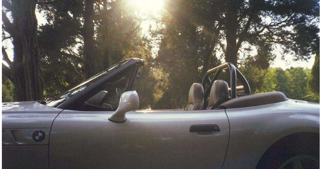
Figure 10 SCCA TTR Spec Roll Bar BMW Z3 Bethania Garage
