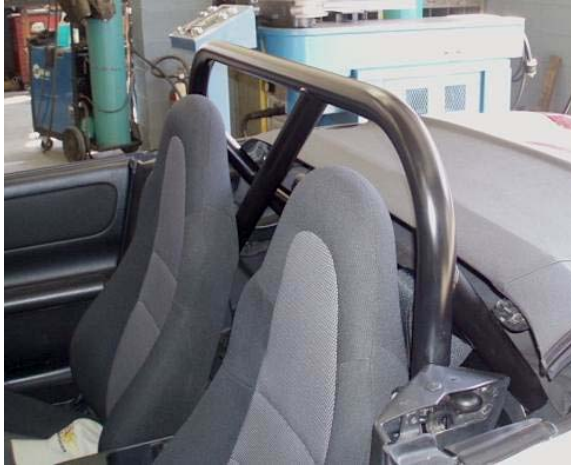
Figure 13 SCCA-TT Spec Roll Bar Toyota MR2 Bethania Garage
