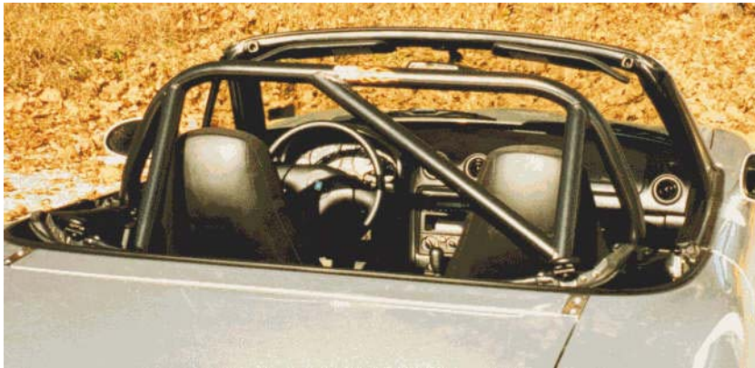
Figure 8 SCCA TTR Spec Roll Bar: "Hard Dog" by Bethania Garage Single Diagonal
