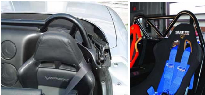
Figure 14 SCCA/NHRA Dodge VIPER Roll Bar #220-601 snakeoylproducts.com Seat lowering Kit #222-532-100-00 required
